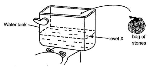
Each time after flushing, water enters and re-fills the tank. The water will stop filling the tank when the water reaches level X.
