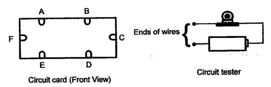
The circuit card was tested with a circuit tester. The ends of the wires of the circuit tester were connected to two points at a time. The table below shows the results.
