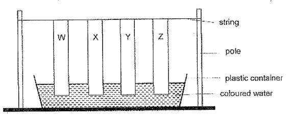
The height in which the coloured water rose to on each strip of material after 5 minutes is recorded in the table below.
