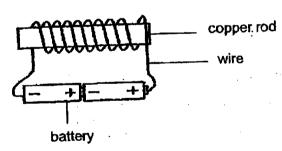
When the electromagnet was brought close to some steel paper clips, none of the paper clips were attracted to it. What could be the reason?
