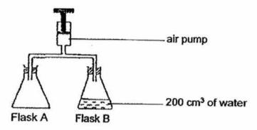
The handle of the air pump is pushed down twice, pushing in 50 cm<sup>3</sup> of air with each pumping action.
