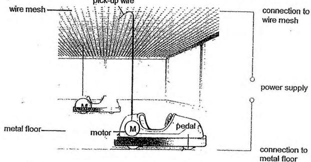
(a) Bumper cars are connected using parallel circuits.
