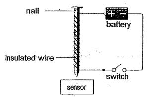
He used a sensor to measure the strength of the electromagnet. He placed the sensor 3 cm from the magnet and increased the number of batteries. He repeated the experiment with the sensor 5 cm from the electromagnet.
