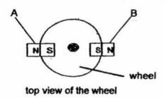
The wheel is fixed to a board in the middle but is able to rotate freely as shown below. The iron bar was attached to a spring that allowed it to move from its original position.
