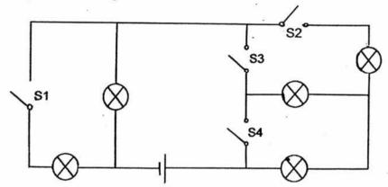
Which pairs of switches will allow only four bulbs to light up when closed?
