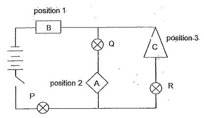
Three different materials, A, B and C, were placed at positions 1, 2 and 3. All the bulbs were identical and functioning properly prior to the experiment.
