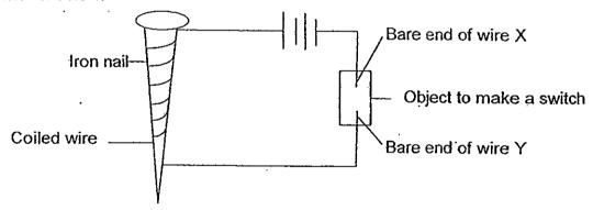
He needed an object to make a switch for the circuit. He wanted to place this object such that it touched the bare ends of wire X and wire Y as shown in the diagram. When he wanted electricity to flow through, he would make both the bare ends of wire X and wire Y touch this object. When he wanted to open the circuit, he would lift the bare end of wire Y such that it would not touch the object.
