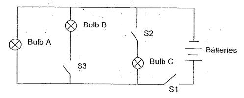
In which order must you close the switches so that Bulb A lights up first, followed by Bulb B and then Bulb C?
