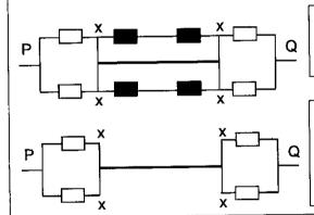
No current passes through the resistors in black as all current will pass through the bold wire (zero resistance).
