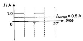
For a single diode rectified sinusoidal current, the mean will be less than 0.5 A as for most of the time the instantaneous current is less than 1.0 A as shown below.
