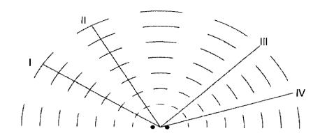
Constructive interference occurs at I, II while destructive interference occurs at III, IV.
