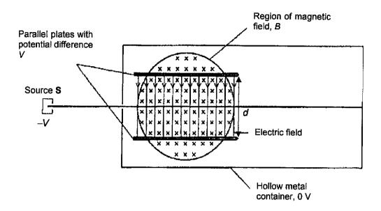
If the potential difference between the parallel plates is V, what is the charge to mass ratio of the ions that can pass through the fields undeflected?
