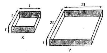
What is the ratio  $\frac{R_X}{R_Y}$  of the resistances between the opposite shaded faces of X and of Y?
