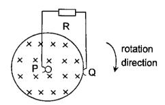
From Fleming left hand rule, electrons at Q will experience a force towards O. Hence Q is at higher potential than P or an induced current will flow from Q to P.
