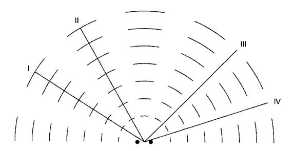
Along which of the labelled lines is the path difference between the waves from the sources equal to  $1.5\lambda$ ?
