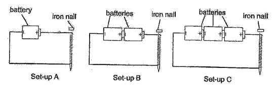
He recorded the number of steel paper clips that each of the magnetised iron nail in set-up A, B and C will attract.
